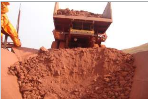
Hopper Feeding By Dumper
